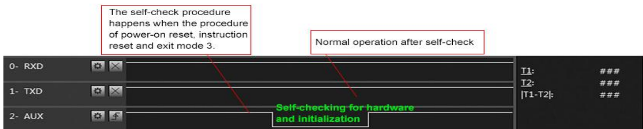
Timing Sequence Diagram of AUX when self-check
